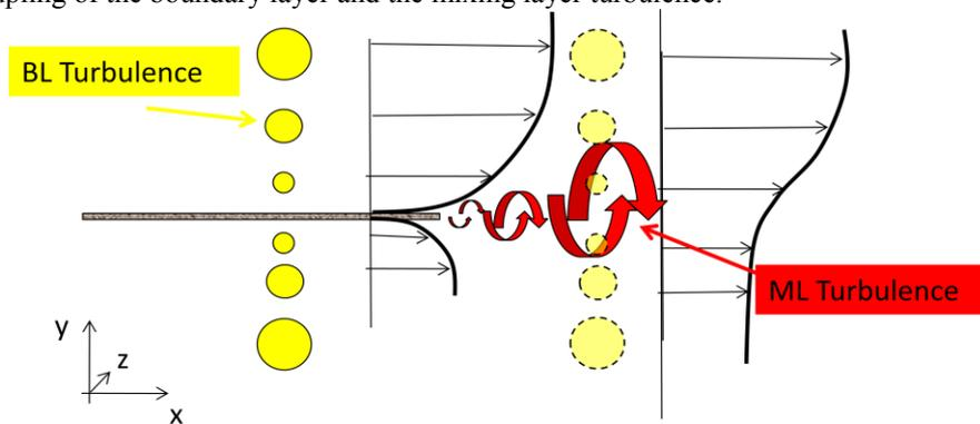
**Figure 5: Generic Mixing length example for locally unstable flows**
