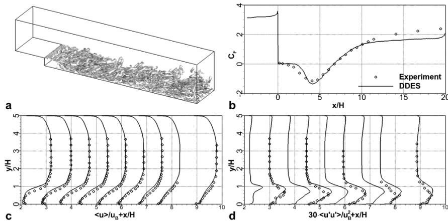
**Figure 6: A sketch of the flow (a) by SST-based DDES: b –skin friction coefficient distribution over the step-wall, c and d – profiles of streamwise velocity  $\langle u \rangle$  and  $\langle u'u' \rangle$  stress, e and f – iso-surfaces of Q criterion equal to 1 [s<sup>-2</sup>]. Profiles are plotted at  $x/H=2.2, 3.0, 3.7, 4.5, 5.2, 5.9, 6.7, 7.4, 8.7$**
