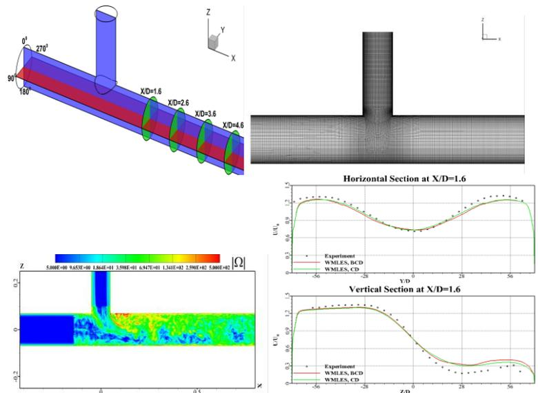
**Figure 7: T-Junction simulation. Upper left: geometry. Upper right: grid. Lower left: turbulence structures. Lower right: axial velocity at station  $X/D=1.6$  for horizontal and vertical lines.**
