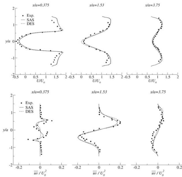
Figure 4: Velocity profiles and turbulence RMS profiles for three different stations downstream of the triangular cylinder ( $x/a=0.375$ ,  $x/a=1.53$ ,  $x/a=3.75$ ). Comparison of SST-SAS, SST-DES models and experiment. (a: U-velocity, b:  $u'v'$ )
