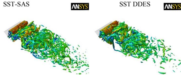
Figure 3: Turbulence structures for flow around triangular cylinder in crossflow.
