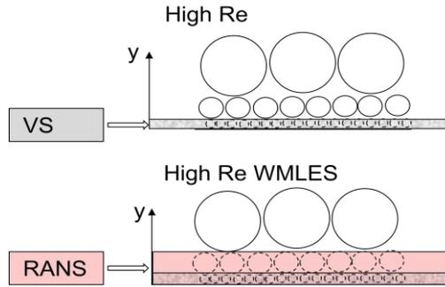
**Figure 1: Concept of WMLES for high  $Re$  number flows. Top: Wall-resolved LES. Bottom: WMLES**
